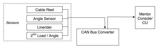
The block diagram tries to clarify that: If the CU does not see any CAN-Bus component, it will report a CAN BUS ERROR.
