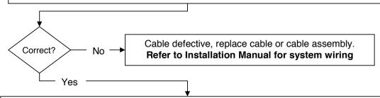
Measure signal from length transducer in cable reel at terminal between pin 2(signal) and pin 1(ground). Retract boom – 0 Potentiometer turn = -0.2V 10 Potentiometer turn = -1.8V.
